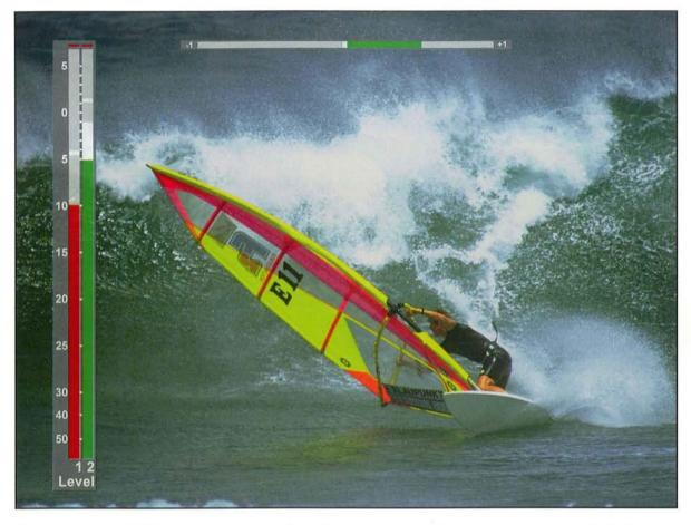
The Chromatec AM-2 is an in-picture and dedicated on-screen audio level meter for displaying two channels of analog or digital audio, in bargraph form.
